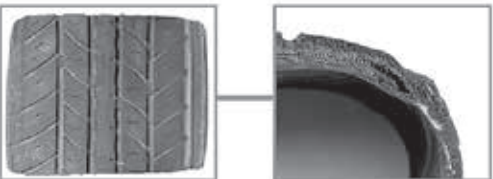
Shoulder Separation - A groove worn in the shoulder of the tire is usually evidence of separation.
