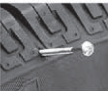
Puncture - Normally, the only evidence of a puncture will be a cut that extends from the tread of the tire through the inner liner.
