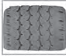
Rapid Shoulder Wear
